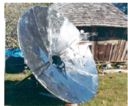
The pot support on this 6' stainless steel dish is attached to a piece of tubing coming up through the center of the dish.
