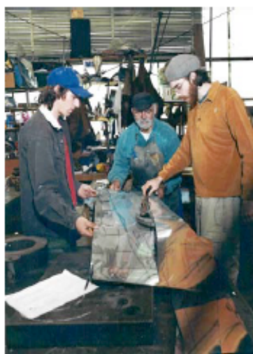
HSU Students using a Beverly shear to cut aluminum sheets into triangular facets.
