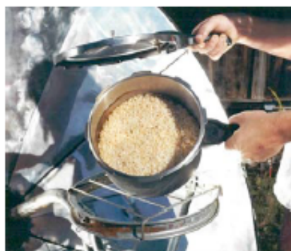
Brown rice cooked in 30 min in a pressure cooker on a parabolic dish.
